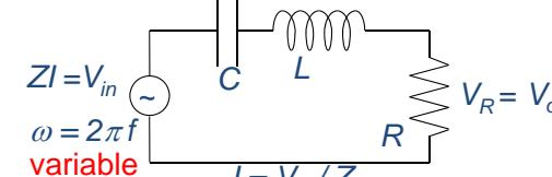
$$H(\omega) = \frac{V_{out}}{V_{in}} = \frac{RI}{ZI} = \frac{R}{\sqrt{R^2 + (L\omega - 1/C\omega)^2}}$$
