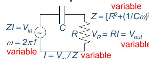
$$H(\omega) = \frac{V_{out}}{V_{in}} = \frac{RI}{ZI} = \frac{R}{\sqrt{R^2 + (1/C\omega)^2}}$$
