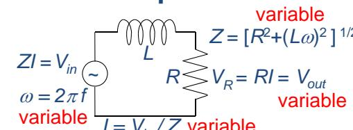
$$H(\omega) = \frac{V_{out}}{V_{in}} = \frac{RI}{ZI} = \frac{R}{\sqrt{R^2 + (L\omega)^2}}$$
